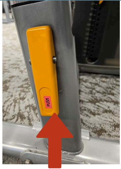
To lower the seat or move the seat farther away, PUSH yellow adjustment lever.
